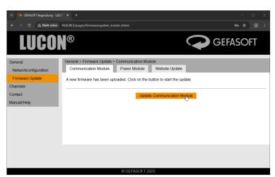
The update will be completed in about 1 minute. During this time the communication controller will be restarted several times.
